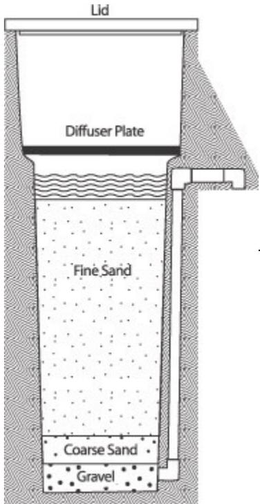
Slow sand filtration has been used for centuries. The filter can be produced locally anywhere in the world because it is built using materials that are readily available. It is simply a concrete container, enclosing layers of sand and gravel whose purpose is to eliminate sediments, pathogens and other impurities from the water. It is in use in over 175,000 homes in over 41 countries around the world.
